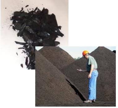
Torrefaction is a thermo-chemical treatment of biomass in the 400 – 650 degree F range. In this process the biomass partly [especially the hemicellulose] decomposes, giving off various types of volatiles.
